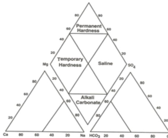
Figure 15: Lozenge field classification of Piper diagram
